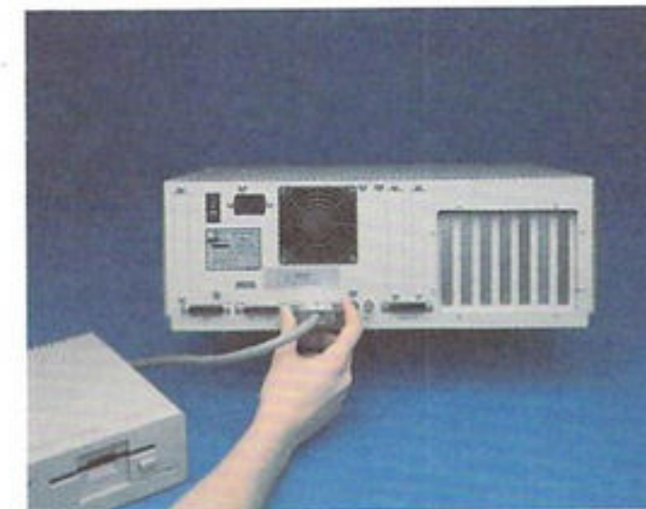
Connecting a 3 1/2-inch disk drive
